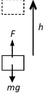
Acceleration of an object raised a distance  $h$  at constant speed = 0, thus  $F$  exerted = weight of the object, i.e.  $F = mg$ .  $WD = Fs = mgh$ . All WD goes into gain in **gravitational potential energy**  $E_p$ , since  $\Delta E_K = 0$ . Therefore,  $E_p = mgh$ .
